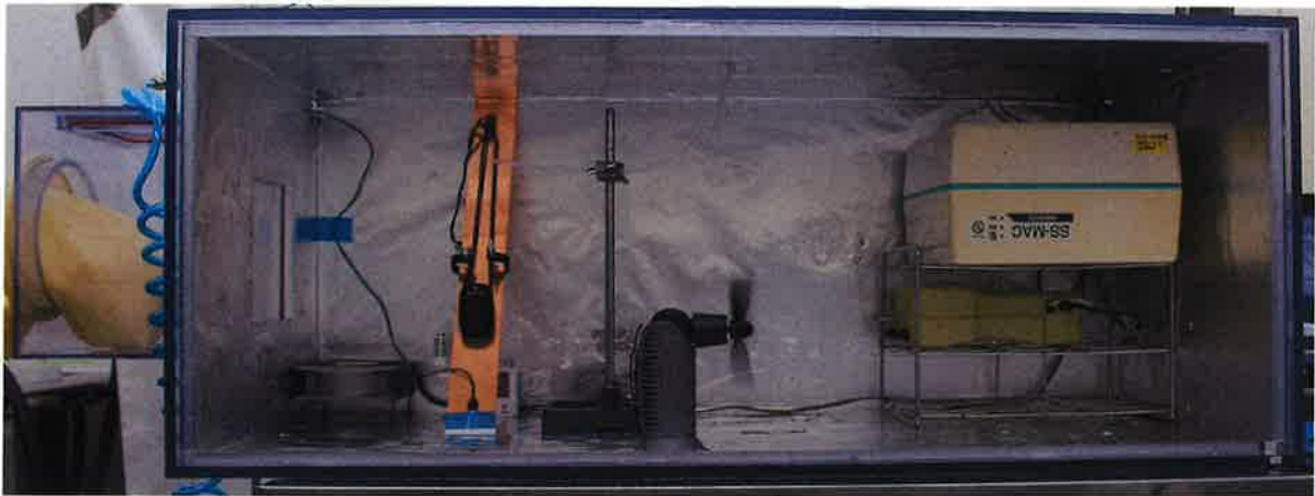
Photo 2. 0.2 m 3 Test chamber (side view) (A315)
